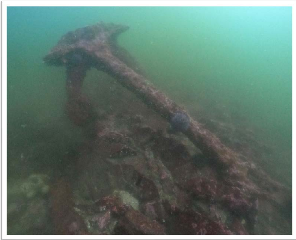
Figure 27. Opposite side view of stockless/patent anchor Target M230829_26 (JL 2023)
